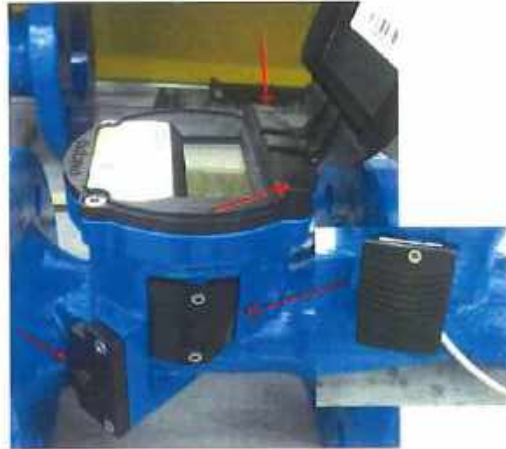
Picture No.7 Emplacement of the seals for security measures
